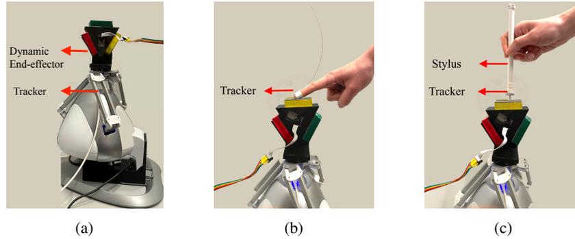
Fig. 1: Our ETHD system, (a) the base of our system is a modified haptic device to render stiffness with a custom dynamic end-effector that is used to render hardness. The user interacts with the end-effector through (b) a bare finger or (c) stylus.
